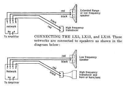
CONNECTING THE N7000 The N7000 dividing network provides a means of adding the 075 to existing high-quality two-way loudspeaker systems to obtain added brilliance in the very high frequencies. It is connected to the high frequency terminals of the main dividing network as shown in the diagrams below:
